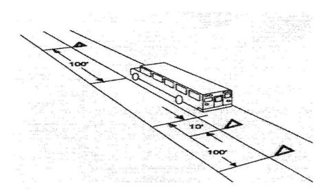
When placing the triangles, hold an assembled triangle toward the oncoming traffic. This enhances safety by increasing visibility to other drivers (especially at night).
